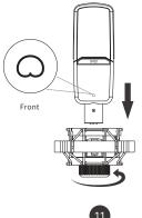
3. Install the included pop filter onto the shock mount as illustrated.
